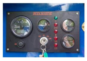
Press the STOP button on the instrument panel.
