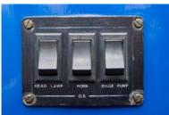
The bilge pumps will operate automatically but can also be operated manually using a switch on the rear deck control console.
