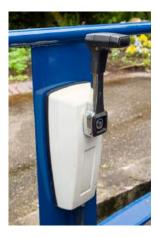
Move the throttle to the upright position and push in the button on the fulcrum of the throttle lever, this disengages the gearbox.
