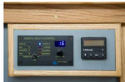
With the engine running above 1200 rpm the boat will provide electrical power (240v a/c) to a maximum load of 1700 watts. Appliances of greater capacity are not permitted.
