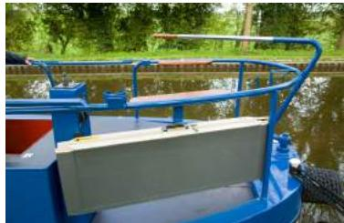
For ease of access there is a metal ramp stored at the rear of the boat. Insert the prongs on the front of the ramp into the holes on the edge of the rear deck.
