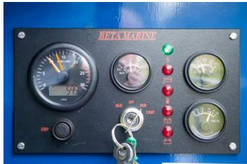
Turn the key anticlockwise to the HEAT position for 6 seconds maximum.
