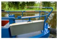
For ease of access there is a metal ramp stored at the rear of the boat. Insert the prongs on the front of the ramp into the holes on the edge of the rear deck.
