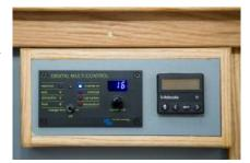
With the engine running above 1200 rpm the boat will provide electrical power (240v a/c) to a maximum load of 2000 watts. Appliances of greater capacity are not permitted.
