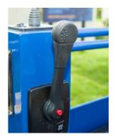
Move the throttle to the upright position and push in the button on the fulcrum of the throttle lever, this disengages the gearbox.
