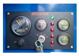
Turn the key anticlockwise to the HEAT position for 6 seconds maximum.
